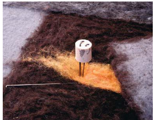
(right) Hand-operated needle felting. Needle felting is the alternative to wet or chemical felting. Industrial needle felting involves machines with hundreds of tiny barbed needles, which push up and down punching and entangling the fibers together. Many nonwoven fabrics are made by needle felting or needle punching.
