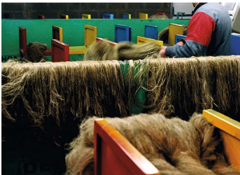
Long fibers (linen flax) processed through a turbine after scutching.
