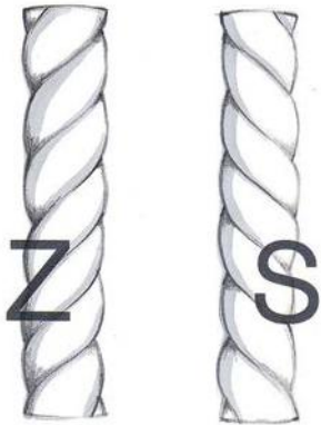
(above) Direction of yarn twist. "Z" twist and "S" twist
