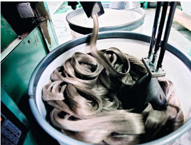
(above) Sliver of flax obtained during drafting and preparation, after combing and before spinning.
