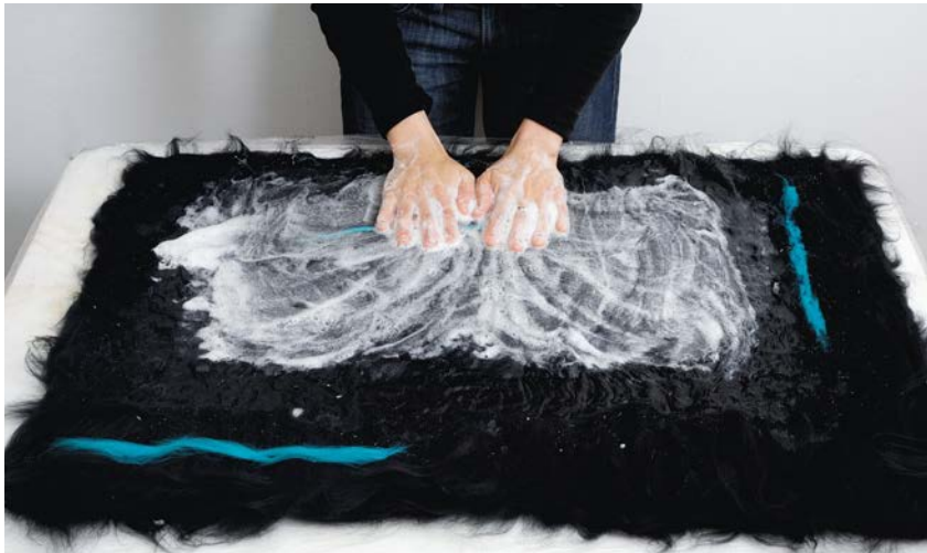
(above) Wet felting. The merino wool fibers are layered at 90 degrees and hot soapy water and friction cause the wool's natural scales to interlock and felt.
